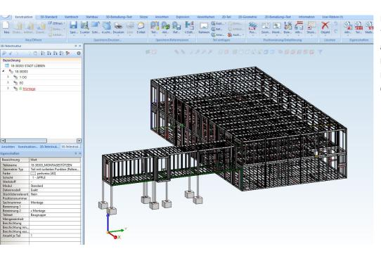
Image: © KLEUSBERG, The complete room modules with a connecting corridor for a school building extension (Nursery & Primary school), in Lübben, Germany (24 modules, 1.200 m<sup>2</sup>) "KLEUSBERG has a competitive edge on the market with regard to working speed due to its modular construction method. HiCAD speeds up the construction through the HCM and parameterization." Ralf Baron, Chief Designer at KLEUSBERG GmbH & Co. KG
